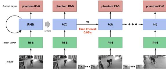
Figure 1: Schematic diagram of the Recurrent Neural Network (RNN) architecture for the autoencoder model. The left side shows the general loop structure of the RNN, and the right side shows its unfolding over time. The input layer (R1-6) receives movie frames, which are processed through the RNN (state  $h(t)$ , weights  $W$ ) to generate reconstructed signals at the output layer (phantom R1-6). The time interval shown is 0.05 s.
